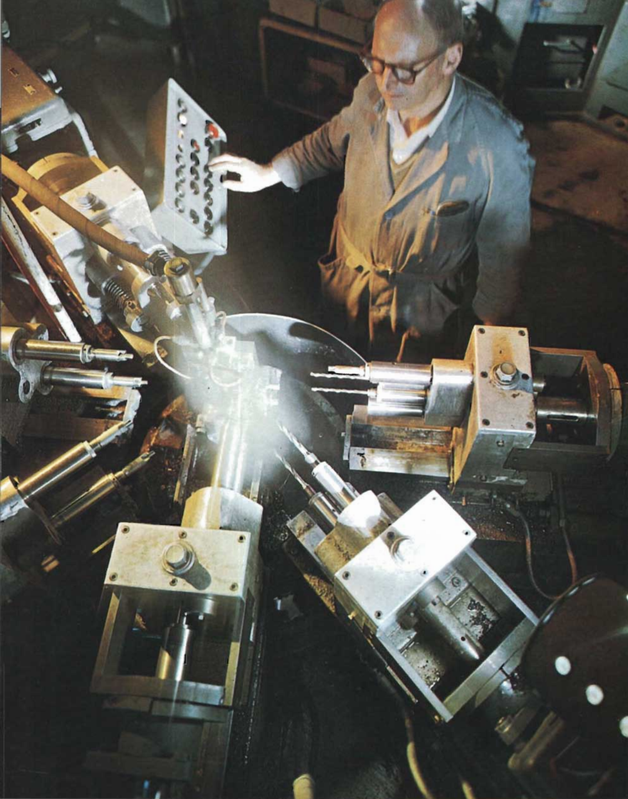
Specialised machining of disc brake calipers. Repco Ltd
