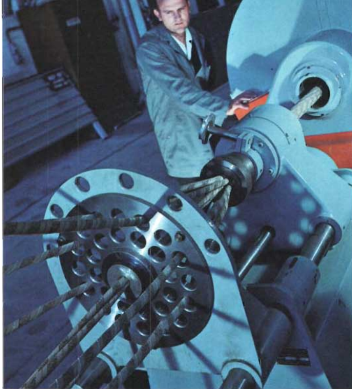
Bundles of quad wire being laid up to form a large telephone cable.
