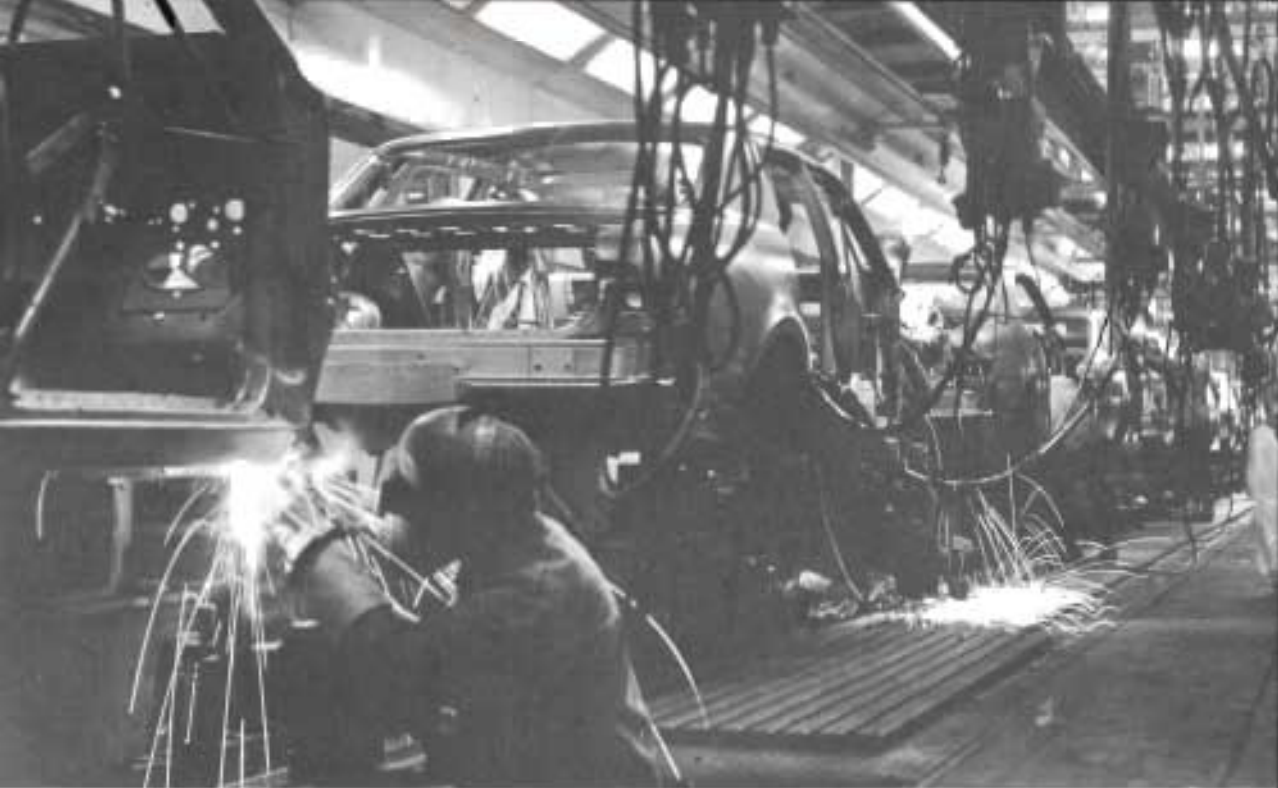
Assembly line production of motor vehicle bodies. General Motors-Holden's Pty Ltd
