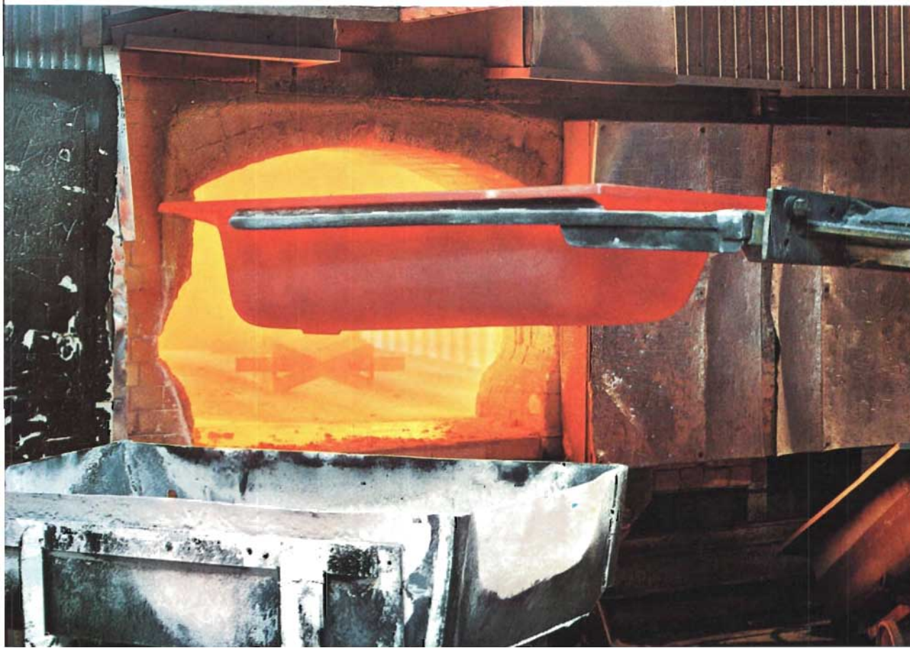
Cast iron bath being removed from heating furnace for enamelling.
